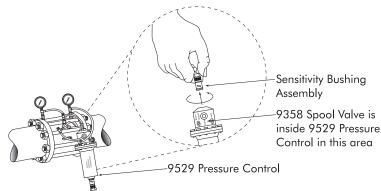
✓ Check the filter to assure it can pass adequate water flow. A partially blocked filter will reduce the valve regulating and closing response time. If little or no flow is present then clean the filter.
