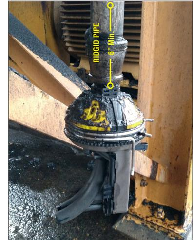
The R75M Debris Sweeping Sprinkler requires a rigid inlet pipe, at least 6" long.
