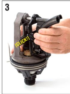
3 Reinstall plate assembly. Guide shift lever between stops as shown in Fig. 4.
