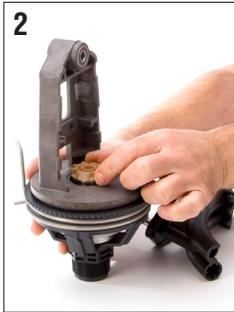
2 Inspect the 7TN nozzle for plugging or damage. Replace if necessary.
