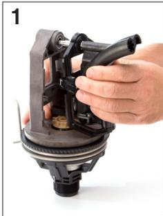
1 Squeeze tabs on the side of the plate assembly and pull.
