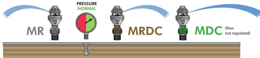
With low pressure, the MR is open, the MRDC and MDC are closed to draining.
