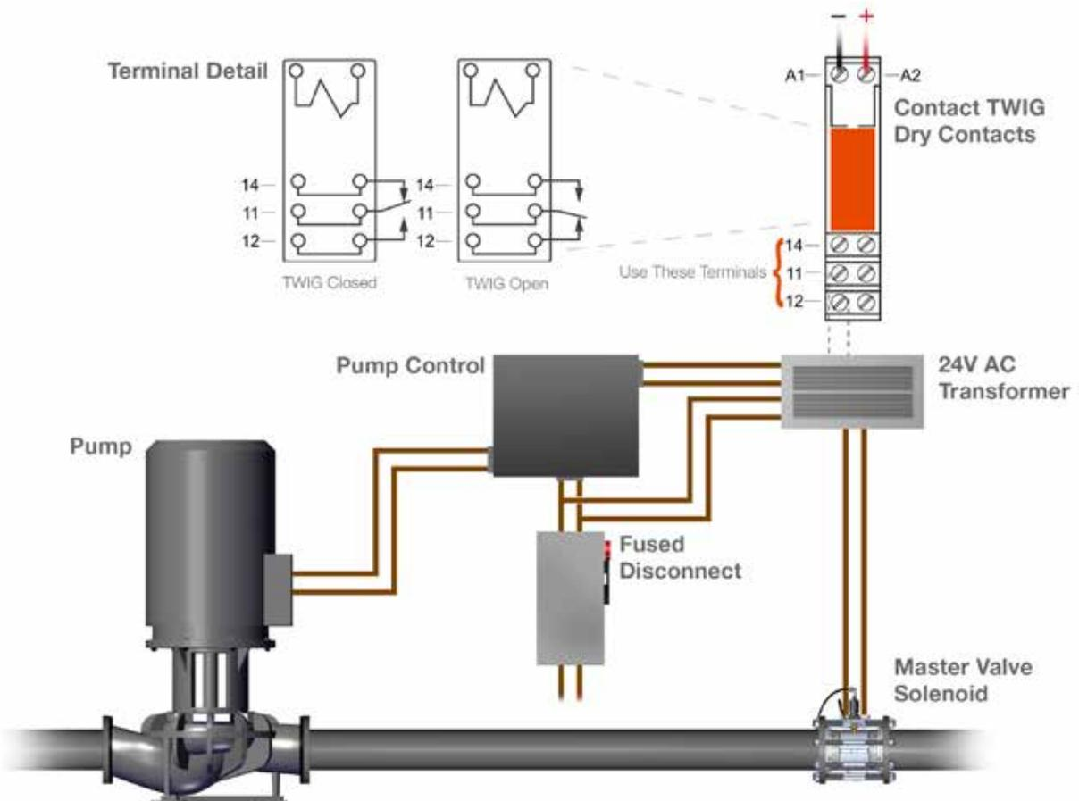
This is a sketch of a typical electric pump layout. In this example one switch is used for the pump and one is used for the master valve. An experienced certified electrician is to make the wiring in conformance with local electrical code).
