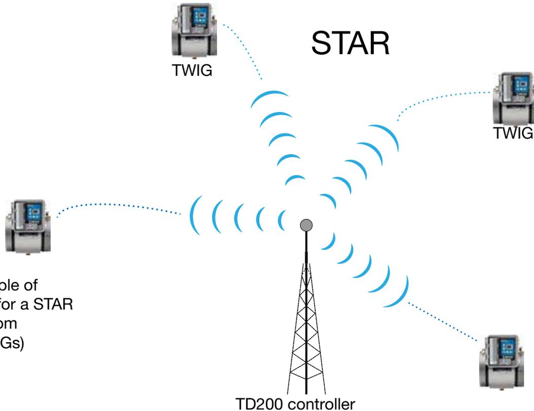
Figure 5.2 Example of communication for a STAR (routing direct from controller to TWIGs)
