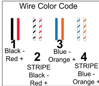
Contact terminals inside the box come pre-wired from the factory. This color chart is simply for reference if a repair is required and to show that the wire polarity is essential.
