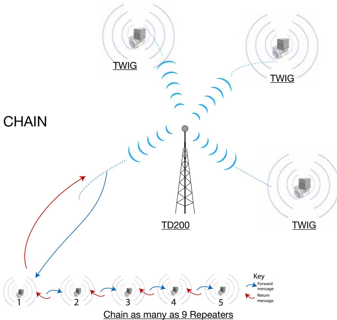
Figure 5.8 Sketch of communication in a Star/Chain combination. The TD200 controller communicates to each TWIG and to the repeaters that are in a chain. Each repeater relays to the next one. This works well to go around problems of signal blockage.
