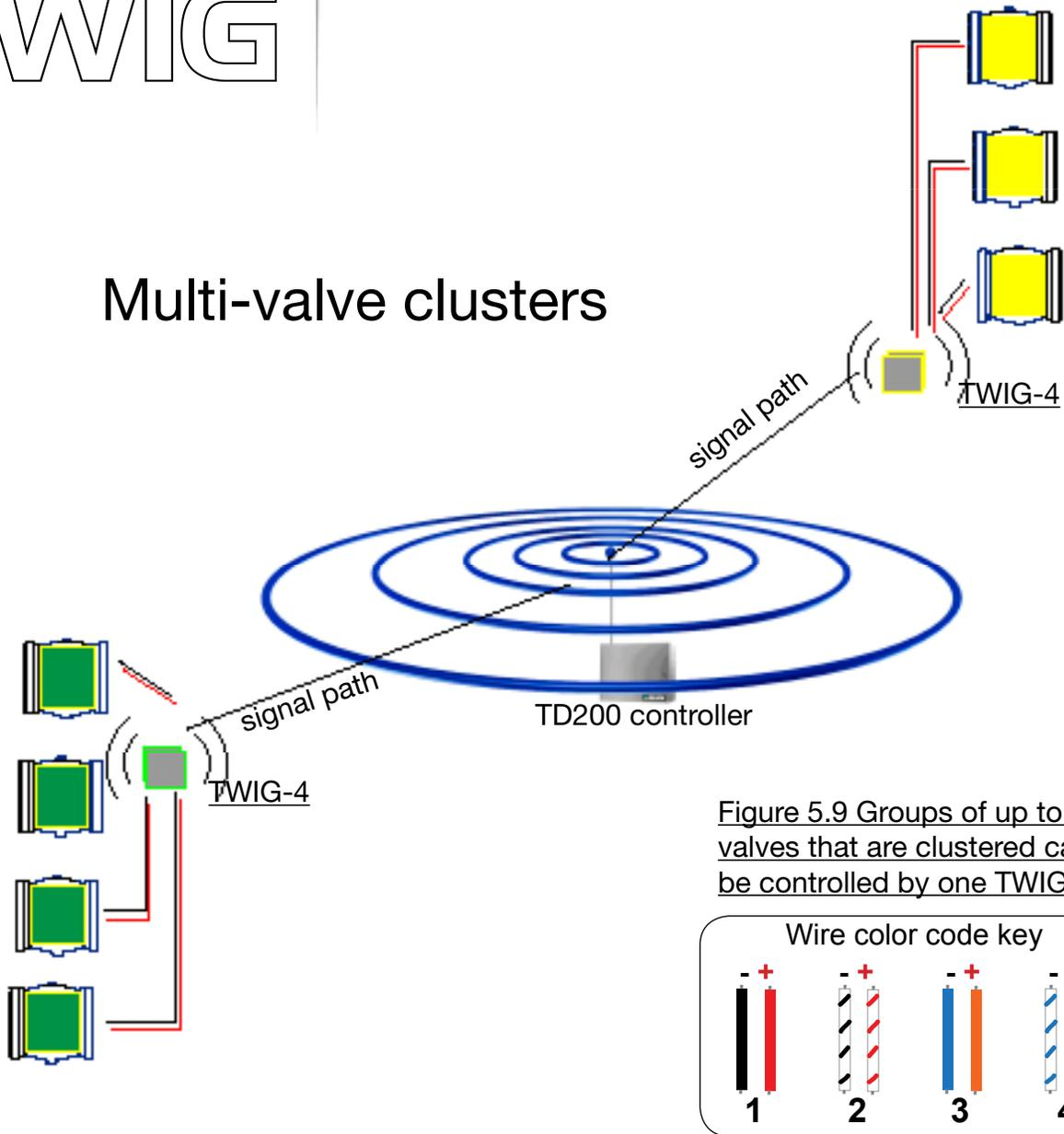
Figure 5.9 Groups of up to four valves that are clustered can be controlled by one TWIG-4.
