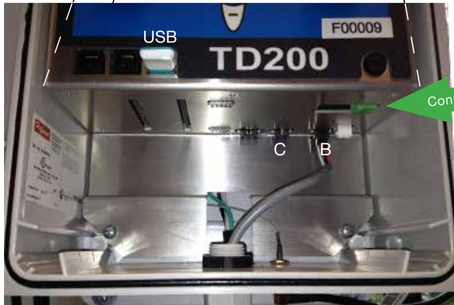
This shows the connection port Conn 1 which is the green port. It can input from a flowmeter or a pause event switch.
