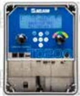
**1** TD200 controller is the foundation of the system and manages the TWIGs on each valve. It includes proprietary Nelson high power radio. Capable of controlling up to 100 TWIGs on valves. The TWIG network has two-way communication every 20 seconds and monitors battery and signal strength for each TWIG valve.
