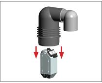
3. Pull float and seal from housing. Clean debris from housing and thoroughly flush before reassembly.
