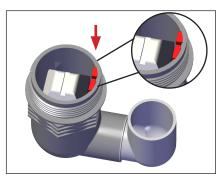
6. Be sure to press the retainer down all the way so that it is even with the housing edge.
