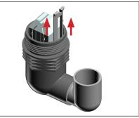
2. Use screwdriver to pry seal retainer out. Pay attention to the correct orientation of the retainer in order to simplify reassembly
