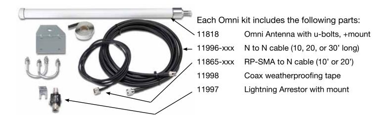
The only difference between these Omni antenna kits is the length of the co-axial antenna cable. The length should be selected carefully because there is some signal degrading within the cable. Length should not be any longer that needed but long enough that it easily connects. An appropriate length will have enough that a small amount of extra cable can be looped to give room for making the connections. The water proof seal tape must be used to keep moisture from entering the cable junctions.
