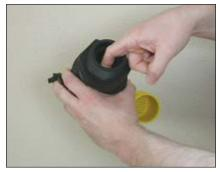
Check to make sure that seal is in place (turn valve upside down, seal should be in place). Finger sweep inside of base (only necessary if valve is used.)
