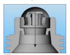
DETAIL 2 Insert seat into valve base.
