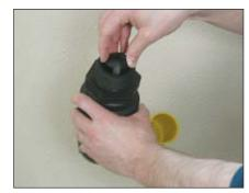
2. Hold valve upside down and place seat (dome up) over hole in base.
