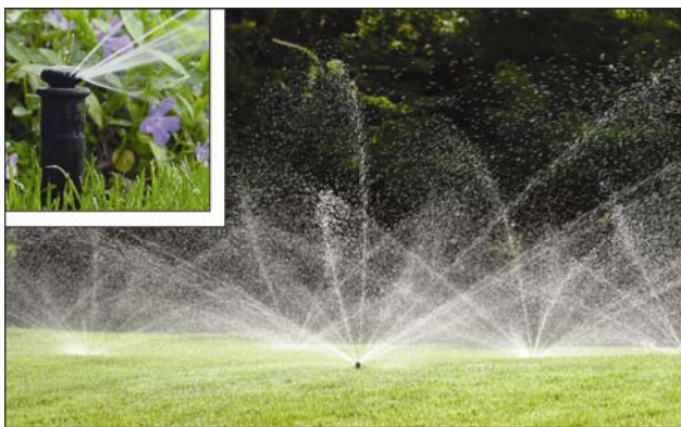
Figure 2. Multi-stream, multi-trajectory rotating (MSMTR) sprinklers. Water leaves the sprinkler in individual streams, which turn slowly, and at multiple trajectory angles (inset) (Photo courtesy of Walla Walla Sprinkler Company).
