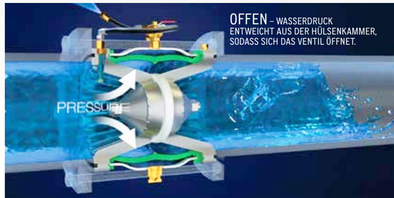
**OFFEN** – WASSERDRUCK ENTWEICHT AUS DER HÜLSENKAMMER, SODASS SICH DAS VENTIL ÖFFNET.
