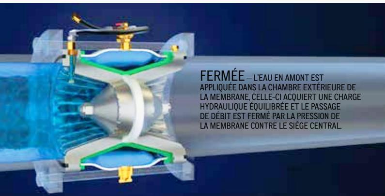
**FERMÉE** – L'EAU EN AMONT EST APPLIQUÉE DANS LA CHAMBRE EXTÉRIEURE DE LA MEMBRANE, CELLE-CI ACQUIERT UNE CHARGE HYDRAULIQUE ÉQUILIBRÉE ET LE PASSAGE DE DÉBIT EST FERMÉ PAR LA PRESSIION DE LA MEMBRANE CONTRE LE SIÈGE CENTRAL.
