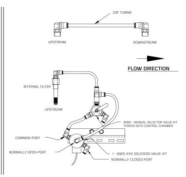
**APPLICATION**: Typical application of the S2 special valve is to connect the valve power to the same power source as the system. If power to the system is off, the solenoid will shut the valve off. Closing the valve will result in a high pressure which can be detected by a high pressure shut-off switch located at the pump. The advantage is no direct electrical connection is required from the valve to the pump.
