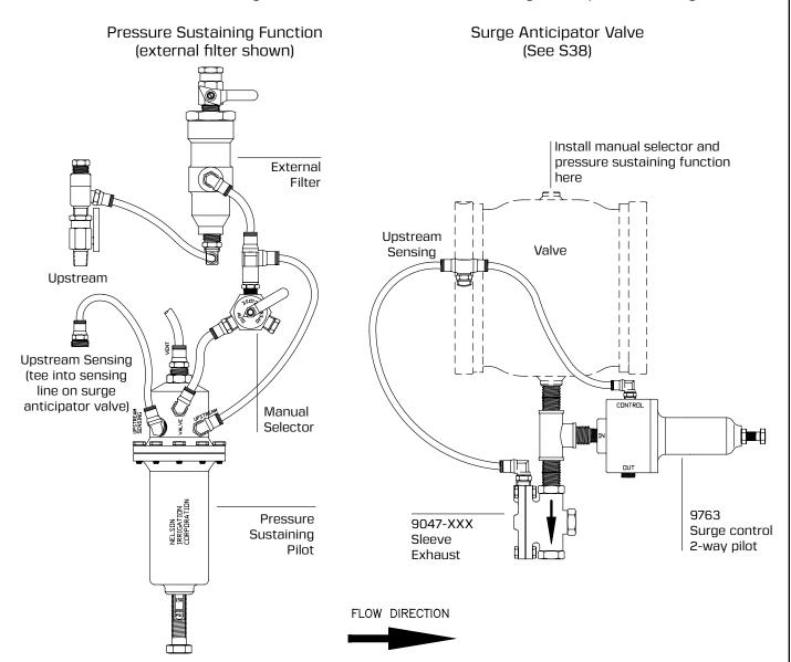
The S50 Valve adds the pressure sustaining function to the S38 Surge Anticipator valve in order to provide a second pressure relief setting. It is set at a value between the D06 Sleeve Exhaust and the 2-way surge control pilot.
