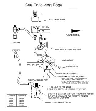
**APPLICATION:** The Nelson control valve with the S31 special deep well application option is used to gradually bring a pump on-line without causing a surge in the mainline system. The manual selector must be put in the "auto" position for the solenoid to work.
