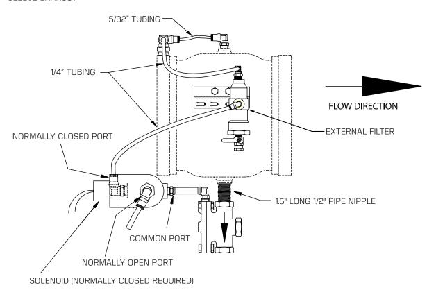
THE SLEEVE EXHAUST NEEDS TO BE ORIENTED NOT ONLY WITH THE FLOW ARROW POINTED OUT OF THE 800 SERIES VALVE, BUT ALSO WITH THE TOP COVER POINTED TOWARDS THE UPSTREAM END OF THE 800 SERIES VALVE. (IF IT IS ORIENTED 90 DEG. TO THIS, THEN IT WILL NOT FIT BETWEEN THE BOLTS IN THE MATING FLANGES DURING FIELD ASSEMBLY.)
