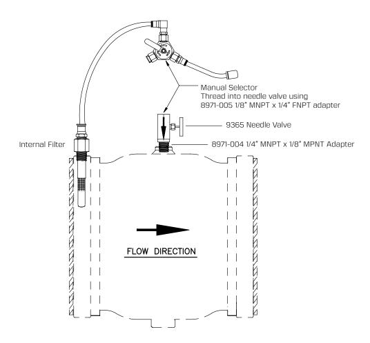
APPLICATION: Typical application of the S1 special valve is for speed control of the valve open/close response. The needle valve on the valve port can be adjusted to set the desired closing and opening response time. Both opening and closing response are affected by the needle valve setting. Closing response time is typically three to six times longer than opening time.
