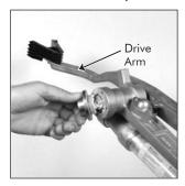
STEP 1 (Drive Arm) Remove four #8311 screws holding #10231 cap. Using an 11/16" socket, remove the #6603 nut from left side of arm.
