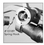
Continue the sequence of sliding onto the drive arm shaft the #10192 spacer and the #10189 spring. Notice the hook end of the spring goes in first so the spring wire loops around the finger of the #10191 cam.
