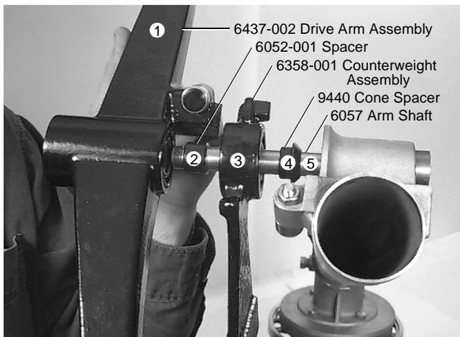
**Figure 9.** Remove components in sequence shown.
