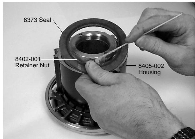
Figure 27. Install seal into housing with lip side facing out.
