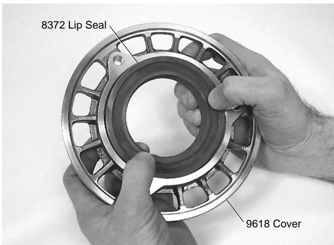
**Figure 24.** With Nelson name toward bearing, install lip seal.
