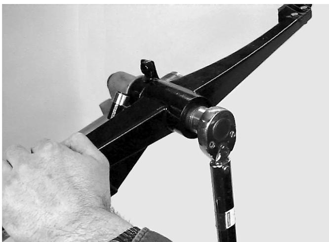
**Figure 15.** Carefully torque arm-shaft nut to prevent damage.
