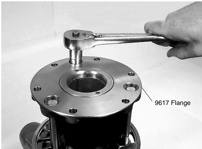
**Figure 29.** Mount flange to lower unit and torque bolts.
