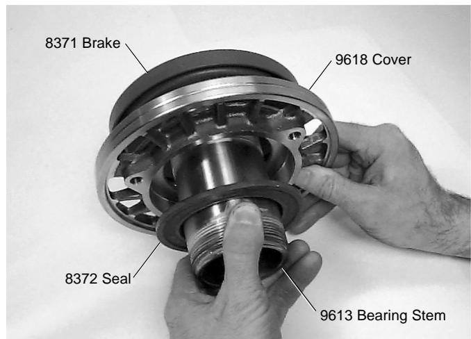
Figure 22. After disassembly, inspect all parts for wear.
