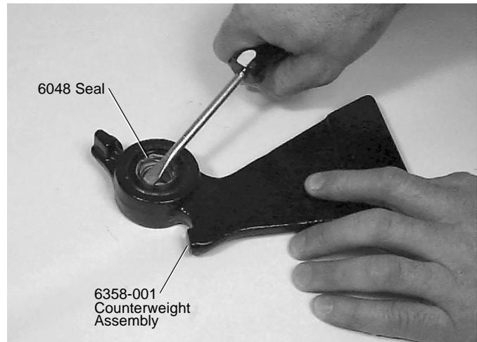
Figure 10. If necessary, remove seals from counterweight.
