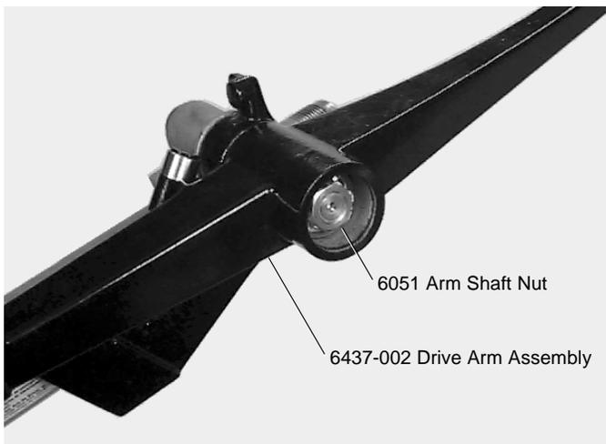
**Figure 8.** Remove arm-shaft nut to remove drive arm.
