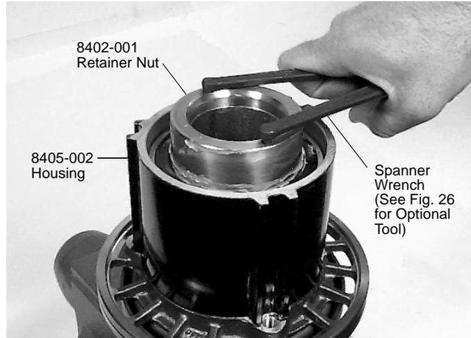
Figure 20. Remove retainer nut using spanner wrench.
