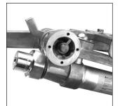
STEP 3 Make sure the #10191 cam is correctly keyed into the slot on the drive arm shaft. Notice the correct orientation of the finger on the cam for proper arm operation.
