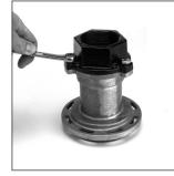
STEP 1 Remove three #6010 screws. Remove 10088-xxx Flange Assembly Connection.
