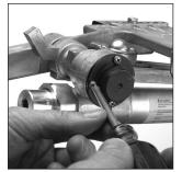
STEP 4 (Drive Arm) Remove four #8311 screws. Remove #10231 cap.
