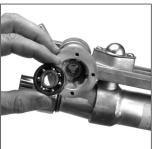
STEP 7 Inspect both left and right #6598 ball bearings. Replace if worn or corroded. Inspect #6600 seals
