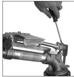
STEP 1 (Trip Lever) Remove two #8311 screws and #10185 cap.
