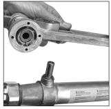
STEP 1 (Shift Lever) Slide #10226-004 shift lever onto mount. Snap the #8323-212 retaining ring onto the mount. Replace the #10364 cap and the two #8311 screws.
