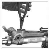
STEP 8 (Shift Lever) Remove two #8311 screws and the #10364 cap. Using retaining ring pliers, remove #8323-212 ring.
