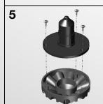
Install new plate by aligning all three holes in the backer plate with the holes in the plate and inserting three screws. Insert plate/motor assembly into body.
