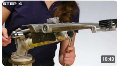
Easily Repair Your Nelson Big Gun Drive Arm With Service Kit 9822 - Step-by-step Tutorial 307 views • 3 weeks ago
