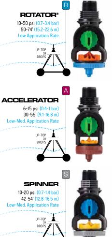
The Rotator' features the greatest throw distance available on drop tubes. The wide water pattern from rotating streams equates to lower average application rates, longer soak time and reduced runoff. More overlap from adjacent sprinklers improves uniformity. 3000 Series (3TN nozzle) or 3030 Series (3NV nozzle).
