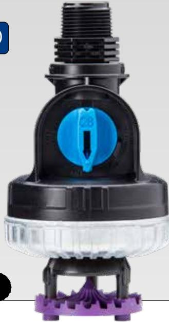
**STREAMLINED DESIGN.** Featuring technology that eliminates the struts of a sprinkler body, Nelson's Pivot Orbitor provides outstanding uniformity and optimal droplets at low pressures (6-20 psi / 0.4-1.4 bar). Expect long wear life and durability in poor water conditions, because there are no sprinkler body struts for debris to hang up on.
