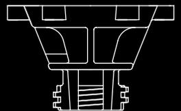
Integral adapter connects directly into all Nelson 3000 & 3030 Series Sprinklers.
