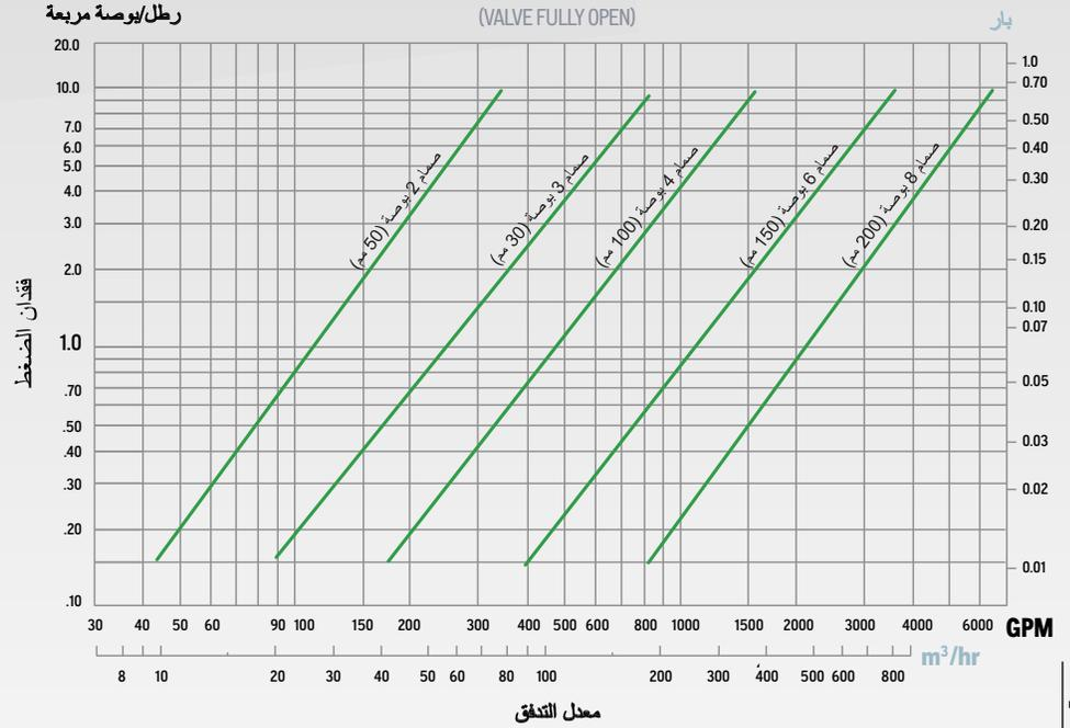
AS A HYDRAULICALLY OPERATED SLEEVE-TYPE VALVE, THE 800 SERIES CONTROL VALVE IS DESIGNED FOR VERSATILITY. THE BASIC BODY CAN BE EQUIPPED WITH SEVERAL DIFFERENT OPTIONS FOR CONTROLLING PRESSURE AND FLOW IN PIPING AT THE PIVOT POINT OR END GUN VALVE CONTROL. IT'S ALSO ENGINEERED FOR EXTREMELY HIGH EFFICIENCY, RESULTING IN LOW PRESSURE LOSS AND HIGH FLOW CAPACITY.
