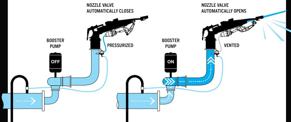
BOOSTER PUMP OFF (EQUAL PRESSURE): DELTA P PRESSURIZES THE LINE LEADING TO THE ACTUATOR ON THE NOZZLE VALVE, MAINTAINING THE VALVE CLOSED.
