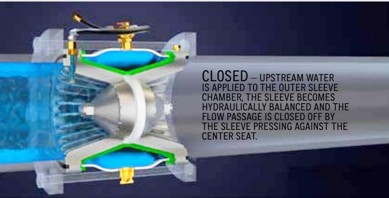
**CLOSED** — UPSTREAM WATER IS APPLIED TO THE OUTER SLEEVE CHAMBER, THE SLEEVE BECOMES HYDRAULICALLY BALANCED AND THE FLOW PASSAGE IS CLOSED OFF BY THE SLEEVE PRESSING AGAINST THE CENTER SEAT.
