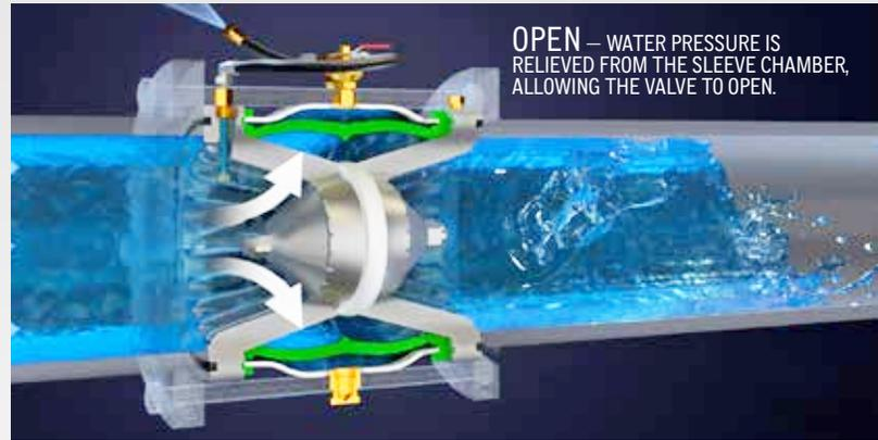
**OPEN** — WATER PRESSURE IS RELIEVED FROM THE SLEEVE CHAMBER, ALLOWING THE VALVE TO OPEN.
