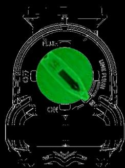
ARROW INDICATES FLOW DIRECTION AND NOZZLE FUNCTION: IN, ON, OFF, FLUSH OR LINE FLUSH
