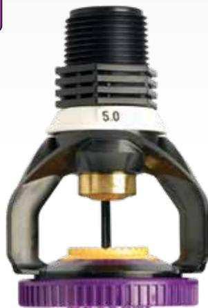
**FLOW CONTROL NOZZLE.** The Flow Control Nozzle (only available for 3000 Series) not only eliminates the need for pressure regulators, but also passes debris more easily. It is not to be used on flexible hose drop assemblies.
