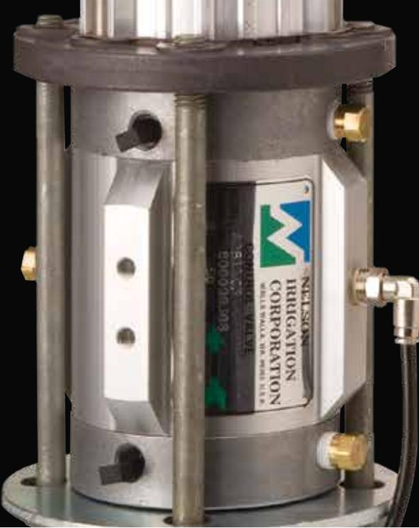
HOW IT WORKS: THE 2" VALVE IS NORMALLY CLOSED. WHEN THE BOOSTER PUMP IS TURNED ON, THE ADDED PRESSURE\* CAUSES THE VALVE TO OPEN OPERATING THE GUN. NO OTHER ACCESSORY IS NEEDED. THE SMALL AMOUNT OF WATER IN THE SLEEVE CHAMBER (ABOUT 1/2 CUP) IS FORCED BACK INTO THE SYSTEM. WHEN THE BOOSTER PUMP IS TURNED OFF THEN THE SYSTEM PRESSURE RE-CLOSES THE VALVE.
