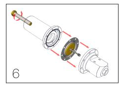
Install the spool assembly in spool housing. Re-assemble the spool housing and the spring housing. Set the adjustment screw to the desired pressure set point.
