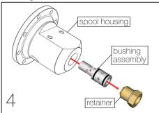
Remove existing bushing assembly. Separate the retainer from the bushing assembly.
