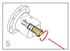
Install the new bushing assembly in the spool housing. Thread-in the retainer.
