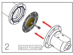
Remove spool assembly from spool housing.
