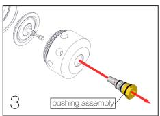
Remove existing bushing assembly from spool housing.
