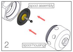
Remove spool assembly from spool housing.
