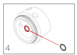
Replace o-ring in spool housing. Careful not to damage o-ring, making sure it is properly seated in the groove.
