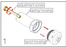
Back-off adjustment screw to remove pressure from the spring. Seperate spring housing from spool housing.
