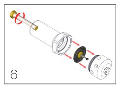
Install the new spool assembly in spool housing. Re-assemble the spool housing and the spring housing. Set the adjustment screw to the desired pressure set point.
