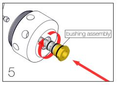
Install the new bushing assembly in the spool housing. Thread-in the retainer.
