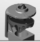
Secure plate/ motor assembly to body by replacing the snap ring.
