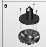
Install new plate by aligning all three holes in the backer plate with the holes in the plate and inserting three screws. Insert plate/motor assembly into body.
