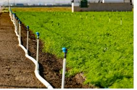
The PC-R2000WF is a Part-Circle Rotator that distributes water in a 180 degree arc. It is intended to irrigate the edge of a field where full circle Rotators are used in the interior.
