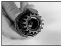
Check inlet and seat area for debris plugging. Remove any debris.
