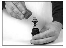
7. A broken plunger/diaphragm assembly can easily be replaced with a new plunger/diaphragm assembly.
