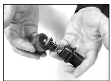
Leakage of water between the cap and housing is an indication of a split plunger.
