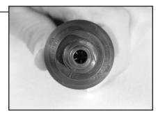
Look in the outlet of the regulator for debris. If cleaning is needed go to 3 below.
