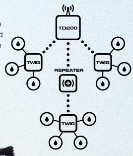
Simply connect Nelson TWIGs to 800 Series Control Valves and couple with the TD200 Controller to automate new or existing drip, solid set or permanent set installations.
