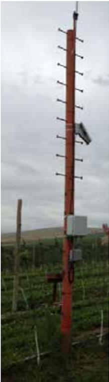
**Repeater:** The TWIG-Repeater is a valuable part of the wireless network. In many fields it is required to extend the range of the radio signals and also to go around obstacles. If electricity is available to power the repeater it is the preferred model to use. For other fields the power must come from solar charged batteries. The repeater is usually mounted on a pole as shown here.
