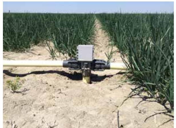
Here are examples of mounting the TWIGs on a stake or a pole. This method provides for going over the top the crop obstructions to get good line-of-sight. The wires from the solenoids must be extended to connect the TWIG wires.
