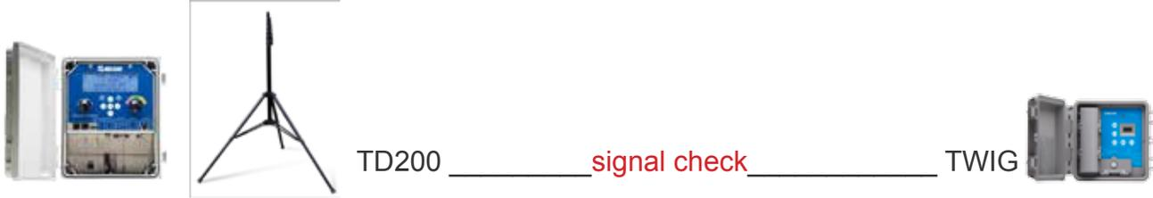
Contact Nelson Irrigation for a source of the aluminum mast support tripods. One antenna mast will be used for the TD200. If the TWIG is to be set high like over tree in an orchard then a second tripod may be necessary and another antenna will be needed. The TWIG-e that can connect to an external antenna will be needed.
