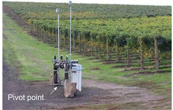
TWIG-2i on a stake in a vineyard. Pivot point to rotate the mast down for access to the TWIG.
