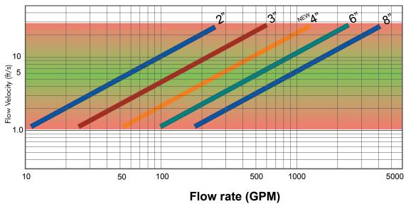
This graph is designed to help select the correct size Nelson 800 Series valve when pressure regulation is needed. To use this graph enter the flow rate axis for the minimum and maximum flows expected. The flow velocity is that estimated for the valve nominal size. Choose the valve size that is within the green band.
