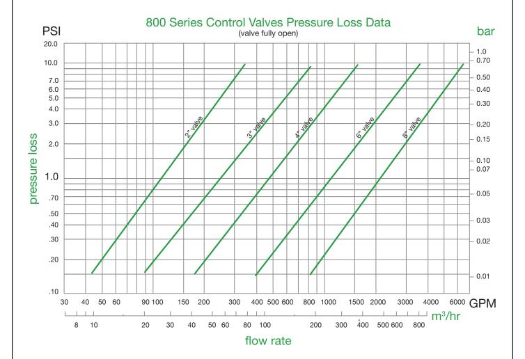
**VALVE SIZE SELECTION NOTE:** In addition to pressure loss, flow velocity must be considered in order to avoid unwanted valve cavitation and pipe sytem water hammer.
