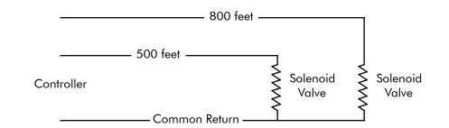
In this example there are two solenoid valves. The first is 500 feet from the controller. The second is a further 300 feet, or a total of 800 feet from the controller. The solenoid valves may be run separately but they may also be run together. The wires need to be designed to meet this flexibility.
